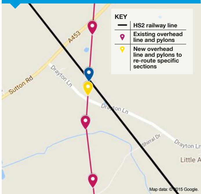
We'll build a new pylon near Drayton Lane, Drayton Bassett, install electricity cable onto it and connect each end to the existing network. The blue marker denotes the location of the pylon being replaced.
