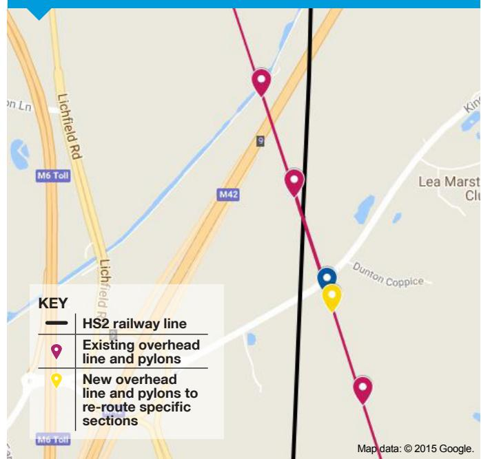
We'll build a new pylon near Dunton Coppice, off Kingsbury Road, install electricity cable onto it and connect each end to the existing network. The blue marker denotes the location of the pylon being replaced.
